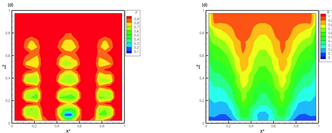
(Left) A plot by MIMPS showing the formation of gas pockets inside fiber tows during PIP; (Right) A MIMPS plot illustrating a complex pattern of temperature distribution inside a PIP mold during processing.
